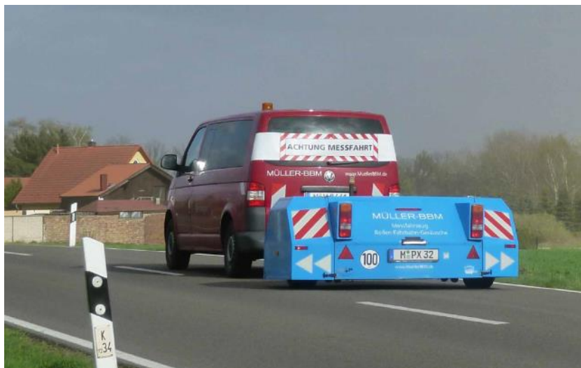
Fig. 20 Example of a CPX system with two test tyres and enclosure (source Müller-BBM)
